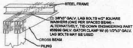
FRAME CONNECTION DETAIL
